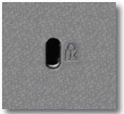
Lock Slot for Locking Cable Harness
